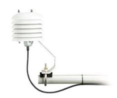
The RAD06 includes a 2 in. U-bolt with a plastic V-block. The U-bolt is placed in the holes on the side of the bracket for attachment to a mast or vertical pole. The U-bolt is placed in the holes on the bottom of the bracket for attachment to a cross-arm.
