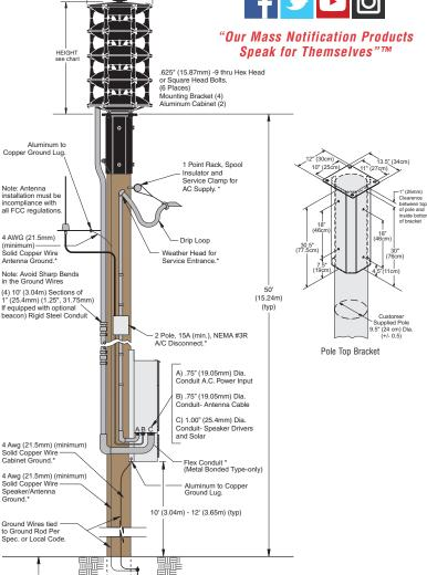
Ground Rods\* Perspec, or Grounding per Local Codes.
