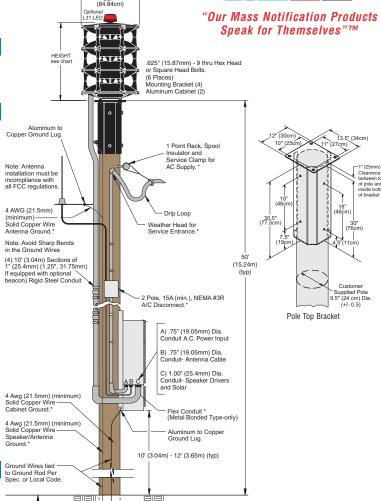
Ground Rods\* Per spec, or Grounding per Local Codes. Customer Supplied
