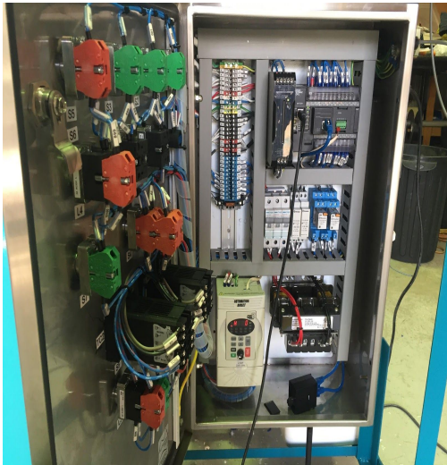
Shruder control system include a: Variable Speed Drive (VSD), Programable Logic Controller (PLC), Wi-Fi connectivity, Safety Switches, Heater Control Units and panel meters.
