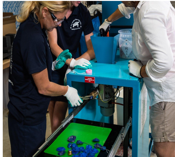
Filament is taken from the extruder and pressed into silicon moulds by the Team at Eco-Barge. The filament can also be drawn onto a spool by the optional spooler with the resulting cord able to be used for handicrafts, 3D printing. Injection moulders can also be attached.
