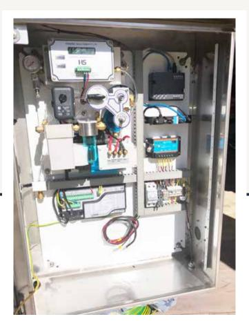
The AWLR-131-BS is a purpose built automatic water level recording system which combines the worlds best data logging equipment, water level sensory equipment and state of the art supporting hardware and software
